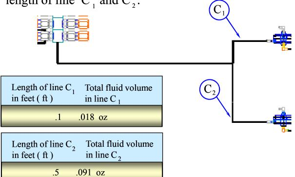
Base upon a single supply pump and line, on Machine #1 for Guns #1 and #2 the length of  $C_1$  and  $C_2$  has been minimized by mounting the regulators and dump valves on the gun bar.
